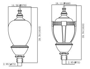
Fixture Body: Die-cast Aluminum
